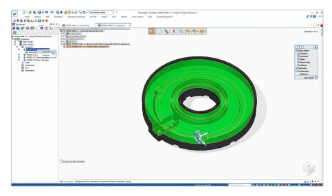
rotation, symmetric and cylindrical variations. The loads are also geometrybased and include mechanical as well as temperature loading for thermal analyses. Mechanical loads include forces, pressures and effects caused by body rotation and gravity. Solid Edge Simulation facilitates load and constraint applications with Quick Bar input options and handles for direction and orientation definition.
